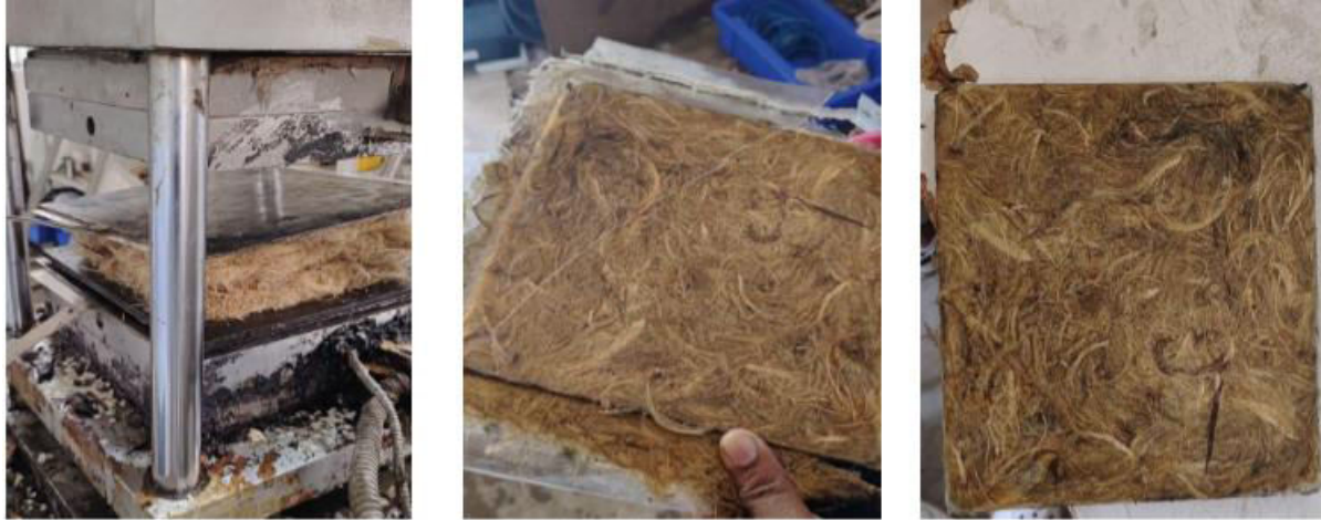
Fig. 4: Fabrication of Arecanut Fibre Reinforced Epoxy Composites
